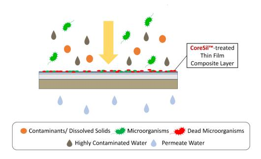
Biofouling Control with CoreSil™ Membrane Technology
